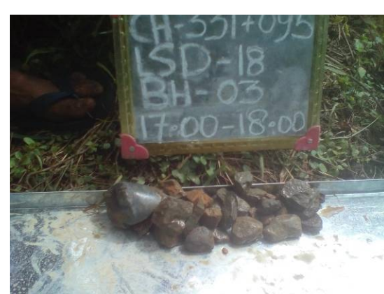
PICTURE 291: BH-3 (Depth-17.00 to 18.00m)
