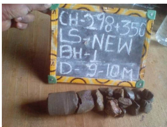
PICTURE 9: BH-1 (Depth-9.00 to 10.00m)
