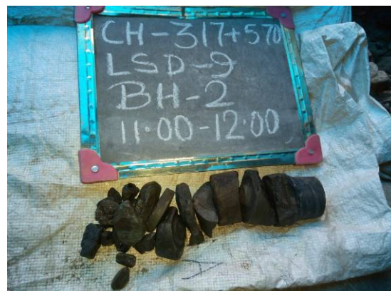
PICTURE 92: BH-2 (Depth-11.00 to 12.00m)
