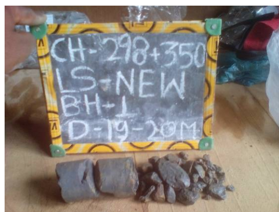
PICTURE 18: BH-1 (Depth-19.00 to 20.00m)
