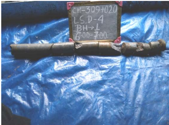
PICTURE 25: BH-1 (Depth-6.00 to 7.00m)
