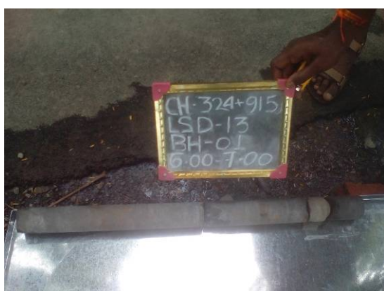
PICTURE 173: BH-1 (Depth-6.00 to 7.00m)
