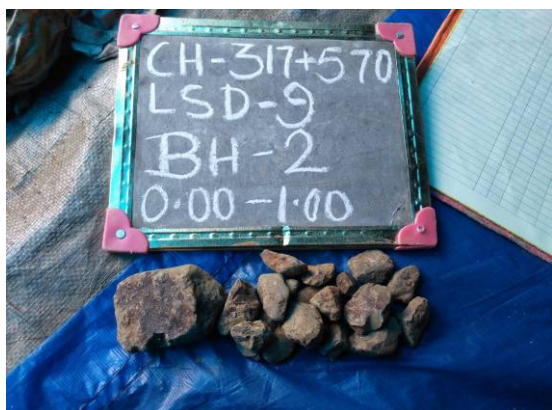
PICTURE 81: BH-2 (Depth-0.00 to 1.00m)
